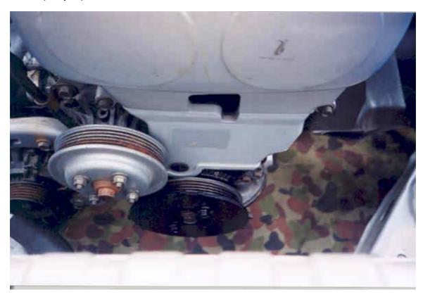
3) The hot water will now exit the engine from the big hole in the head just below the #1 intake port (check photo 3). Also the water intake is now on the RWD water pump which you already fitted 'right. We'll get back to this later
